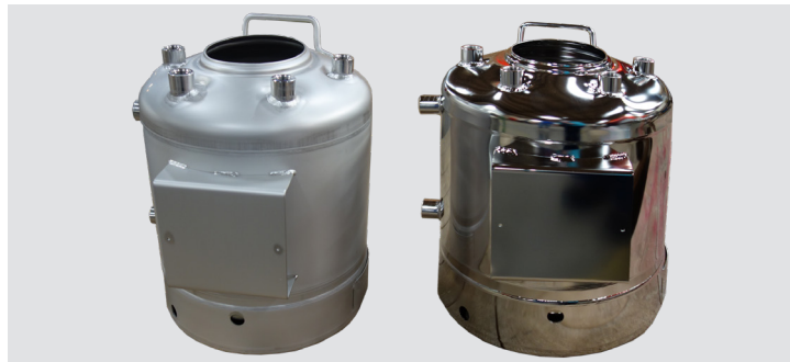
These vessels in different stages of the finishing process measure 17.34 RA on the pickle passivation sample (left) and 7.92 RA after pickle passivation and electropolishing (right).
