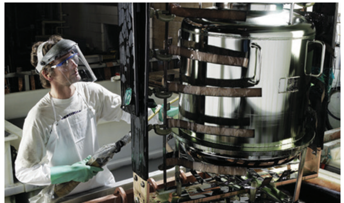
A hygienic industry portable vessel emerges from the electro-polishing tank at Apache Stainless Equipment Corporation.
